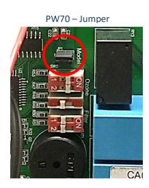
3. Ozone settings can be adjusted by manipulating the dipswitches located on the PCB. \* DEFAULT SETTINGS
